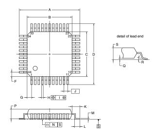
NOTE Each lead centerline is located within 0.16 mm of its true position (T.P.) at maximum material condition
